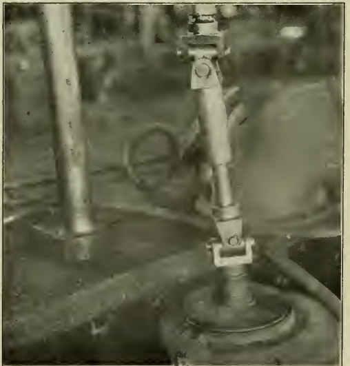
Fig. 4—A Method of Grinding Throttle Valves by Power.
